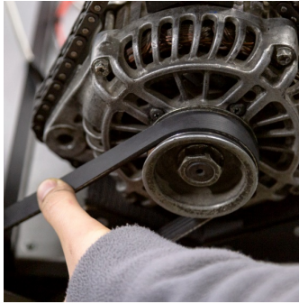
Figure 17. Belt tightness check
